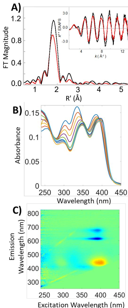
**Figure 2:** A) A comparison of the non-phase shift corrected Fourier Transforms of the Hg L3-edge EXAFS data for 1:1 (—) and 2:1 (—) mixtures of mb-SB2:Hg<sup>2+</sup>. The inset shows the corresponding EXAFS comparison. B) Absorbance spectra of mb-SB2 titrated with 10 0.1 equivalents of Hg<sup>2+</sup>. C) Difference fluorescence excitation- emission matrix of mb-SB2 and a 1:1 mixture of mb-SB2 and Hg<sup>2+</sup>.
